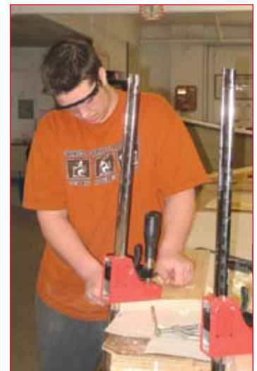
Josh uses a spokeshave to chamfer a seat for the boat.
